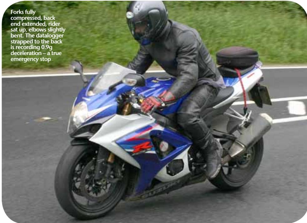
Forks fully compressed, back end extended, rider sat up, elbows slightly bent. The datalogger strapped to the back is recording 0.9g deceleration – a true emergency stop
