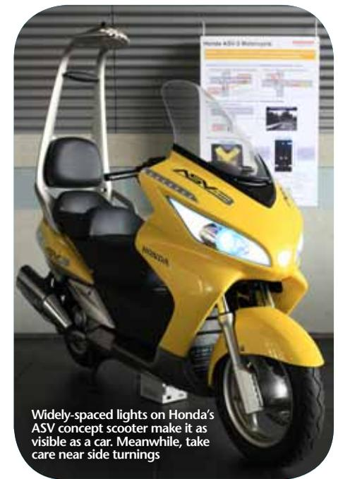
Widely-spaced lights on Honda's ASV concept scooter make it as visible as a car. Meanwhile, take care near side turnings
